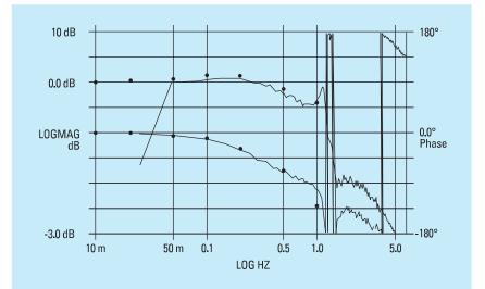
Figure 1A: Comparing DSA and stepped-sine testing In this test on a generator operating at 246 MW, the DSA measurement clearly shows a local mode between 1.0 and 1.1 Hz. The stepped sine measurement (represented by the eight gain and phase points) missed this critical information
